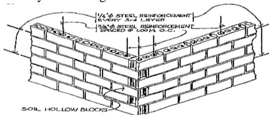
Hollow concrete block masonry (Source: Google images)
