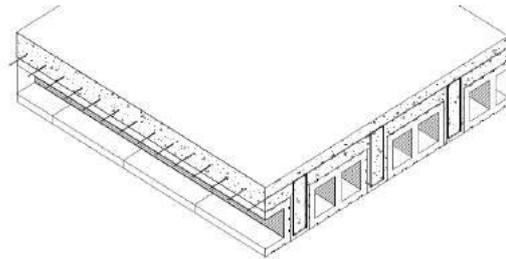
Filler slab using Hollow concrete block
