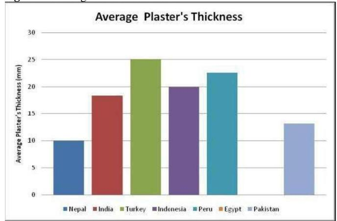
Figure 9. Average Plaster's Thickness
