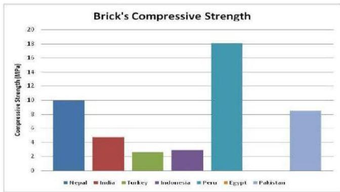
Figure 8. Brick Compressive Strength
